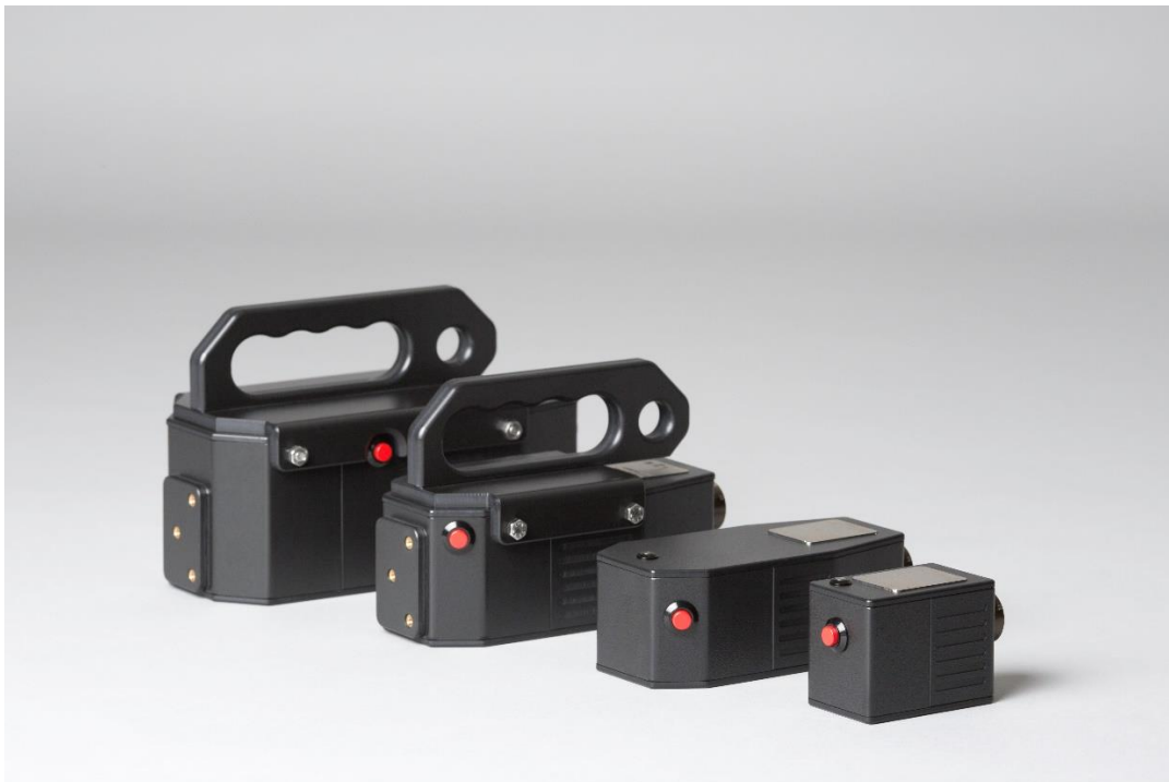
Four standard probes: small, medium, large and extra-large, each optimized for a specific lift-off range. The software assists the operator to select the best probe for each application.
