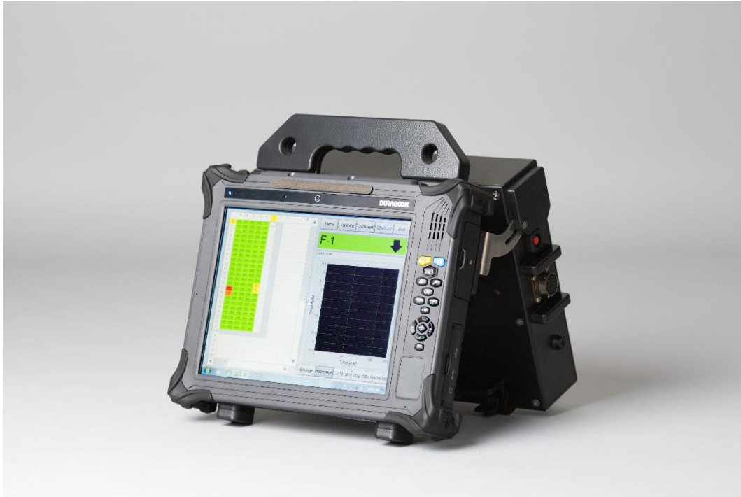
PECT instrument, showing data acquisition tablet computer that is permanently attached to a data acquisition and pulse generating unit. Instrument operation is from a touch screen.
