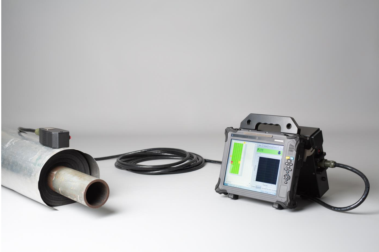
The PECT instrument connected to a probe with a 8m long signal cable
